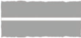
Stop line at signals or police control
