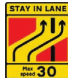
One lane crossover at contraflow road works
