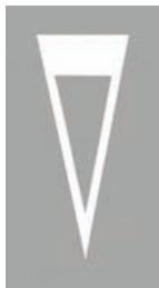
Warning of 'Give Way' just ahead
